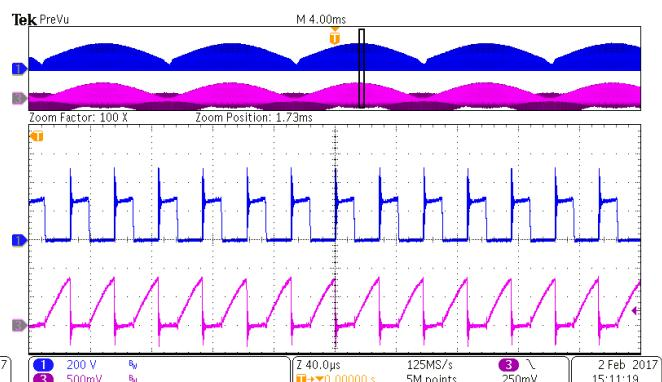
Fig. 15 Drain & CS waveforms @ 90Vac/60Hz/Zoom-In
