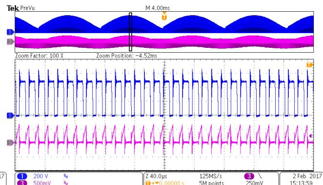
Fig. 19 Drain & CS waveforms @ 230Vac/50Hz/Zoom-In
