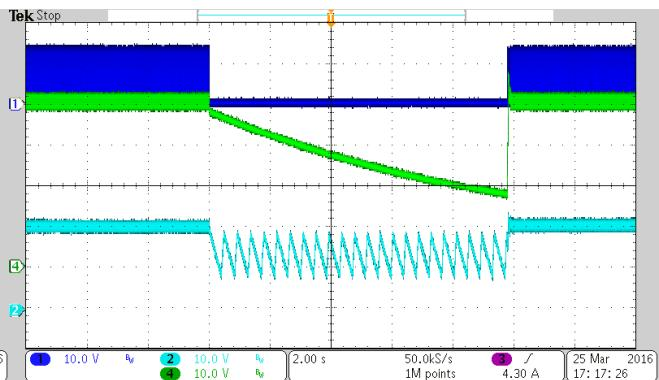
Fig. 13 Over Temp. Protection @ 264Vac/50Hz
