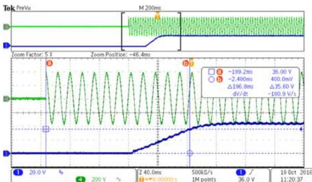
Fig. 4 Start-up Waveforms @ 90V<sub>ac</sub>/60Hz
