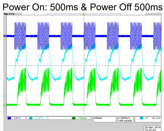
Fig. 22 AC On/Off Test @ 90Vac/60Hz
