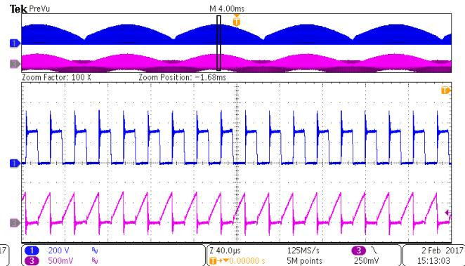
Fig. 17 Drain & CS waveforms @ 115Vac/60Hz/Zoom-In
