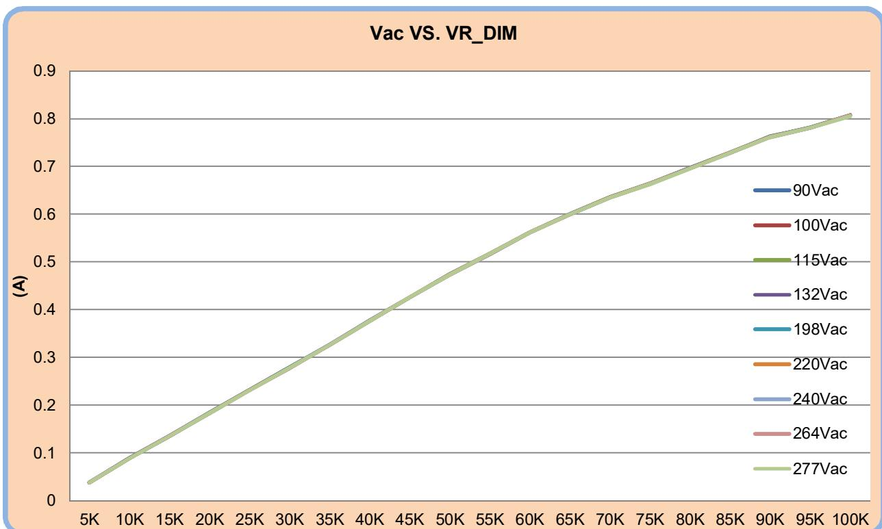
Fig. 25 Dimming performance test at full range
