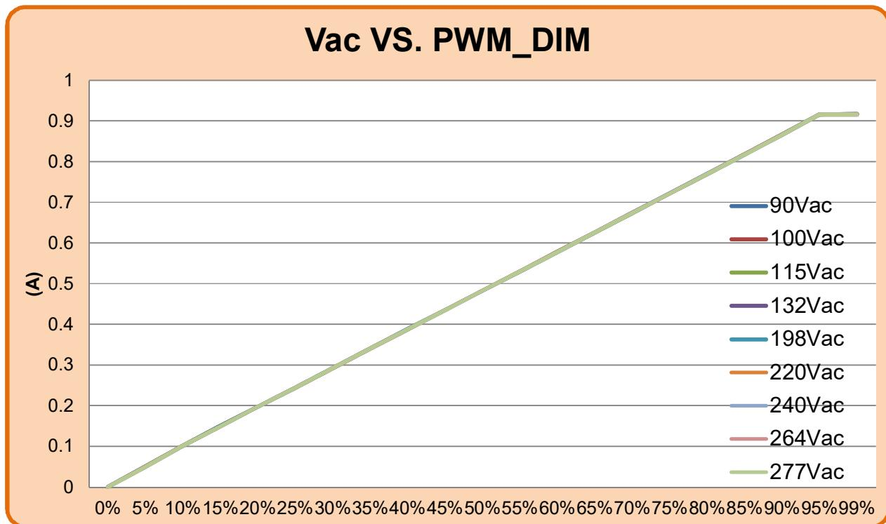
Fig. 24 Dimming performance test at full range
