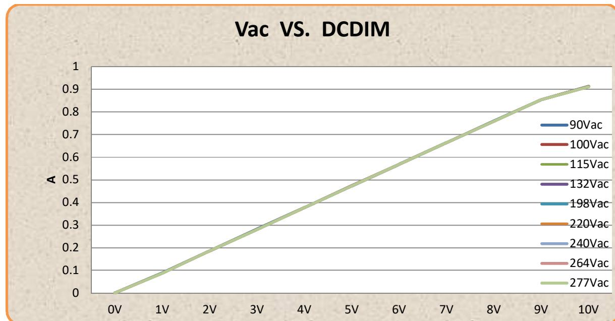
Fig. 23 Dimming performance test at full range
