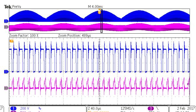
Fig. 21 Drain & CS waveforms @ 264Vac/50Hz/Zoom-In
