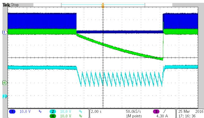
Fig. 12 Over Temp. Protection @ 90Vac/60Hz
