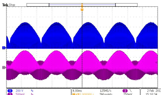
Fig. 14 Drain & CS waveforms @ 90Vac/60Hz
