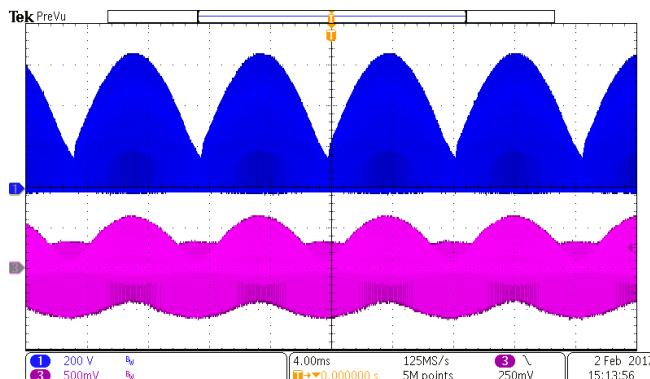
Fig. 18 Drain & CS waveforms @ 230Vac/50Hz
