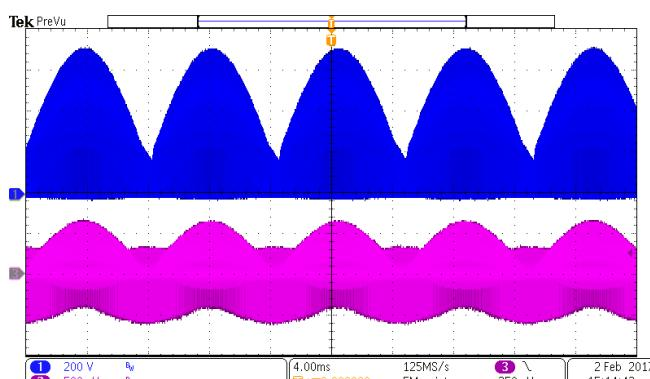
Fig. 20 Drain & CS waveforms @ 264Vac/50Hz
