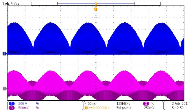
Fig. 16 Drain & CS waveforms @ 115Vac/60Hz
